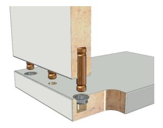
Cabinets are glued together without a cabinet press or clamps. Assembly is carried out as usual with wooden dowels, with an additional DÜBELKLEMME being used for every 2nd or 3rd dowel to bridge the curing time of the glue.
